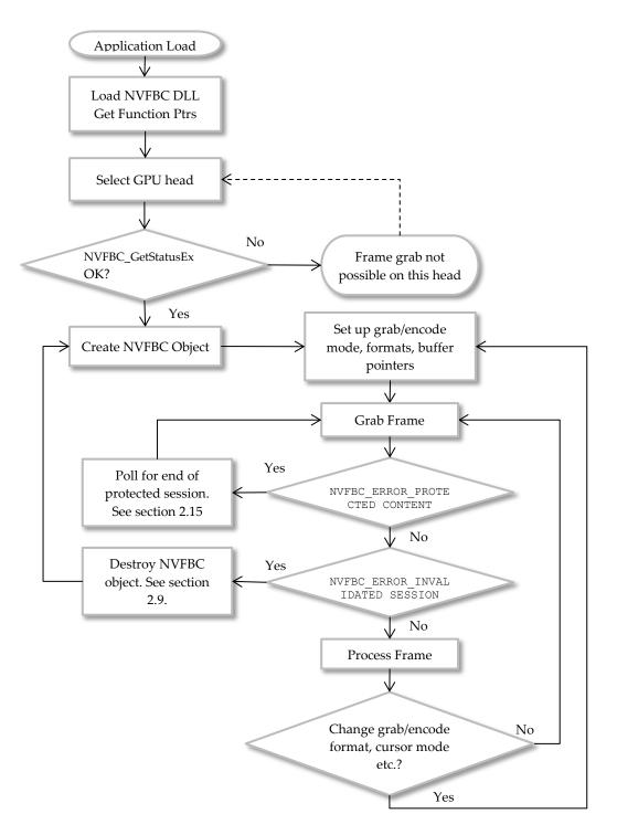
Figure 2 Overview of NVFBC application flow
